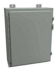
Hammond enclosure, NEMA 12/13, 20 x 16 x 6in (HxWxD), wall mount, carbon steel, ANSI 61 gray, powder coat finish, single-door, stainless steel clamps, padlock hasp and staple.
