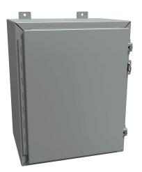
Hammond enclosure, NEMA 12/13, 20 x 16 x 12in (HxWxD), wall mount, carbon steel, ANSI 61 gray, powder coat finish, single-door, stainless steel clamps, padlock hasp and staple.
