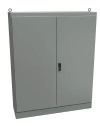
Hammond enclosure, NEMA 12, 90 x 72 x 24in (HxWxD), freestanding, dual access, carbon steel, ANSI 61 gray, powder coat finish, double-door, 3-point keylocking handle.
