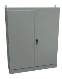
Hammond enclosure, NEMA 12, 90 x 72 x 24in (HxWxD), freestanding, carbon steel, ANSI 61 gray, powder coat finish, double-door, 3-point keylocking handle.
