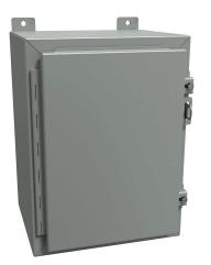
Hammond enclosure, NEMA 12/13, 16 x 12 x 10in (HxWxD), wall mount, carbon steel, ANSI 61 gray, powder coat finish, single-door, stainless steel clamps, padlock hasp and staple.
