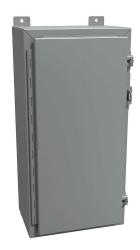
Hammond enclosure, NEMA 12/13, 24 x 12 x 8in (HxWxD), wall mount, carbon steel, ANSI 61 gray, powder coat finish, single-door, stainless steel clamps, padlock hasp and staple.
