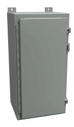
Hammond enclosure, NEMA 12/13, 24 x 12 x 10in (HxWxD), wall mount, carbon steel, ANSI 61 gray, powder coat finish, single-door, stainless steel clamps, padlock hasp and staple.
