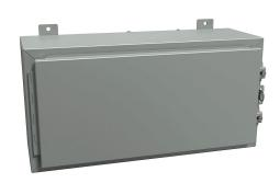
Hammond enclosure, NEMA 12/13, 12 x 24 x 8in (HxWxD), wall mount, carbon steel, ANSI 61 gray, powder coat finish, single-door, stainless steel clamps, padlock hasp and staple.
