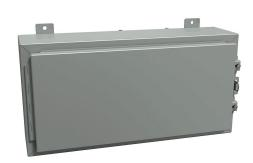
Hammond enclosure, NEMA 12/13, 12 x 24 x 6in (HxWxD), wall mount, carbon steel, ANSI 61 gray, powder coat finish, singledoor, stainless steel clamps, padlock hasp and staple.
