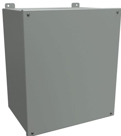
Hammond enclosure, NEMA 12/13, 16 x 14 x 8in (HxWxD), wall mount, carbon steel, ANSI 61 gray, powder coat finish, screw cover.
