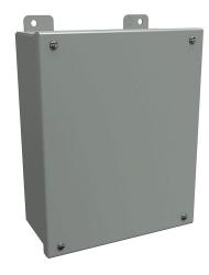
Hammond enclosure, NEMA 12/13, 10 x 8 x 4in (HxWxD), wall mount, carbon steel, ANSI 61 gray, powder coat finish, screw cover.
