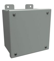
Hammond enclosure, NEMA 12/13, 6 x 6 x 4in (HxWxD), wall mount, carbon steel, ANSI 61 gray, powder coat finish, screw cover.
