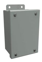
Hammond enclosure, NEMA 12/13, 6 x 4 x 3in (HxWxD), wall mount, carbon steel, ANSI 61 gray, powder coat finish, screw cover.
