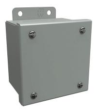
Hammond enclosure, NEMA 12/13, 4 x 4 x 3in (HxWxD), wall mount, carbon steel, ANSI 61 gray, powder coat finish, screw cover.
