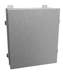
Hammond enclosure, NEMA 3R/4/4X/12/13, 14 x 12 x 6in (HxWxD), wall mount, 304 stainless steel, #4 brush finish, lift-off cover, stainless steel clamps.
