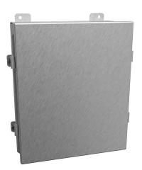
Hammond enclosure, NEMA 3R/4/4X/12/13, 12 x 10 x 5in (HxWxD), wall mount, 304 stainless steel, #4 brush finish, lift-off cover, stainless steel clamps.
