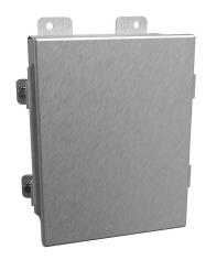
Hammond enclosure, NEMA 3R/4/4X/12/13, 8 x 6 x 3.5in (HxWxD), wall mount, 304 stainless steel, #4 brush finish, lift-off cover, stainless steel clamps.
