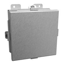
Hammond enclosure, NEMA 3R/4/4X/12/13, 6 x 6 x 4in (HxWxD), wall mount, 304 stainless steel, #4 brush finish, lift-off cover, stainless steel clamps.
