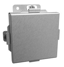
Hammond enclosure, NEMA 3R/4/4X/12/13, 4 x 4 x 3in (HxWxD), wall mount, 304 stainless steel, #4 brush finish, lift-off cover, stainless steel clamps.
