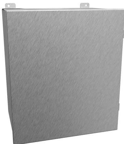
Hammond enclosure, NEMA 3R/4/4X/12/13, 16 x 14 x 10in (HxWxD), wall mount, 304 stainless steel, #4 brush finish, single-door, stainless steel clamps.
