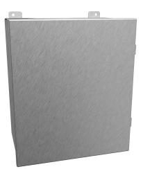
Hammond enclosure, NEMA 3R/4/4X/12/13, 14 x 12 x 8in (HxWxD), wall mount, 304 stainless steel, #4 brush finish, single-door, stainless steel clamps.
