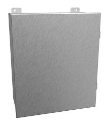
Hammond enclosure, NEMA 3R/4/4X/12/13, 14 x 12 x 6in (HxWxD), wall mount, 304 stainless steel, #4 brush finish, single-door, stainless steel clamps.
