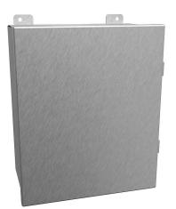
Hammond enclosure, NEMA 3R/4/4X/12/13, 12 x 10 x 6in (HxWxD), wall mount, 304 stainless steel, #4 brush finish, single-door, stainless steel clamps.
