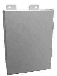
Hammond enclosure, NEMA 3R/4/4X/12/13, 8 x 6 x 3.5in (HxWxD), wall mount, 304 stainless steel, #4 brush finish, single-door, stainless steel clamps.
