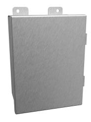
Hammond enclosure, NEMA 3R/4/4X/12/13, 8 x 6 x 4in (HxWxD), wall mount, 304 stainless steel, #4 brush finish, single-door, stainless steel clamps.
