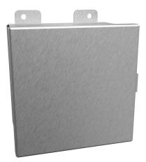
Hammond enclosure, NEMA 3R/4/4X/12/13, 6 x 6 x 4in (HxWxD), wall mount, 304 stainless steel, #4 brush finish, single-door, stainless steel clamps.
