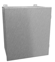
Hammond enclosure, NEMA 3R/4/4X/12/13, 16 x 14 x 10in (HxWxD), wall mount, 316 stainless steel, #4 brush finish, single-door, stainless steel clamps.
