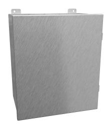
Hammond enclosure, NEMA 3R/4/4X/12/13, 14 x 12 x 8in (HxWxD), wall mount, 316 stainless steel, #4 brush finish, single-door, stainless steel clamps.
