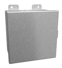
Hammond enclosure, NEMA 3R/4/4X/12/13, 6 x 6 x 4in (HxWxD), wall mount, 316 stainless steel, #4 brush finish, single-door, stainless steel clamps.
