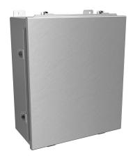
Hammond enclosure, NEMA 4/4X/12/13, 14 x 12 x 6in (HxWxD), wall mount, 5052-H32 aluminum, lift-off cover, aluminum clamps.
