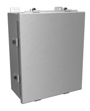
Hammond enclosure, NEMA 4/4X/12/13,  $12 \times 10 \times 5$ in (HxWxD), wall mount, 5052-H32 aluminum, lift-off cover, aluminum clamps.
