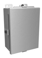
Hammond enclosure, NEMA 4/4X/12/13, 8 x 6 x 3.5in (HxWxD), wall mount, 5052-H32 aluminum, lift-off cover, aluminum clamps.
