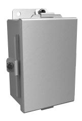
Hammond enclosure, NEMA 4/4X/12/13, 6 x 4 x 3in (HxWxD), wall mount, 5052-H32 aluminum, lift-off cover, aluminum clamps.
