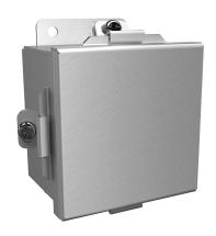
Hammond enclosure, NEMA 4/4X/12/13,  $4 \times 4 \times 3$ in (HxWxD), wall mount, 5052-H32 aluminum, lift-off cover, aluminum clamps.
