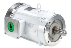
Leeson Washguard White Duck premium efficiency AC induction motor, washdown and inverter rated, 7-1/2hp, 3-phase, 230/460 VAC, 1800rpm, TEFC, NEMA 213TC frame, rolled steel, C-face mount.
