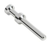
METE crimp contact, male, 16 amp, accepts wire size 20 AWG, silver-plated copper alloy. Package of 100. For use with METE multi-wire male inserts rated for 16 amps.
