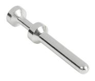
METE crimp contact, male, 16 amp, accepts wire size 26-22 AWG, silver-plated copper alloy. Package of 100. For use with METE multi-wire male inserts rated for 16 amps.
