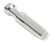
METE crimp contact, female, 16 amp, accepts wire size 16 AWG, silver-plated copper alloy. Package of 100. For use with METE multi-wire female inserts rated for 16 amps.
