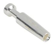
METE crimp contact, female, 16 amp, accepts wire size 20 AWG, silver-plated copper alloy. Package of 100. For use with METE multi-wire female inserts rated for 16 amps.
