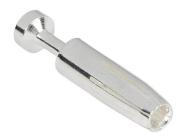
METE crimp contact, female, 16 amp, accepts wire size 26-22 AWG, silver-plated copper alloy. Package of 100. For use with METE multi-wire female inserts rated for 16 amps.
