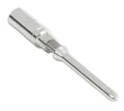
METE crimp contact, male, 10 amp, accepts wire size 14 AWG, silver-plated copper alloy. Package of 100. For use with METE multi-wire male inserts rated for 10 amps.
