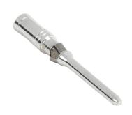
METE crimp contact, male, 10 amp, accepts wire size 16 AWG, silver-plated copper alloy. Package of 100. For use with METE multi-wire male inserts rated for 10 amps.
