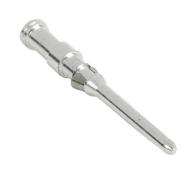
METE crimp contact, male, 10 amp, accepts wire size 18 AWG, silver-plated copper alloy. Package of 100. For use with METE multi-wire male inserts rated for 10 amps.
