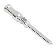
METE crimp contact, male, 10 amp, accepts wire size 26-22 AWG, silver-plated copper alloy. Package of 100. For use with METE multi-wire male inserts rated for 10 amps.
