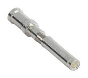
METE crimp contact, female, 10 amp, accepts wire size 16 AWG, silver-plated copper alloy. Package of 100. For use with METE multi-wire female inserts rated for 10 amps.
