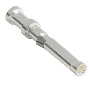
METE crimp contact, female, 10 amp, accepts wire size 20 AWG, silver-plated copper alloy. Package of 100. For use with METE multi-wire female inserts rated for 10 amps.
