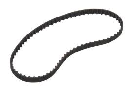
SureMotion timing belt, 1/5in XL pitch, 1/4in wide, 70 tooth, 14in pitch length (circumference), neoprene, fiberglass reinforced.
