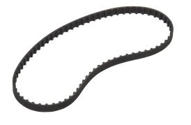
SureMotion timing belt, 1/5in XL pitch, 1/4in wide, 70 tooth, 14in pitch length (circumference), neoprene, fiberglass reinforced.
