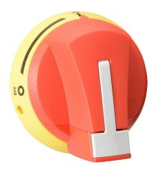
Socomec rotary handle, round, S01, red/yellow, external front or right side mount, 2-position, lockable in OFF only, defeatable, NEMA 1/3R/12.
