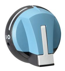
Socomec rotary handle, round, S01, black/blue, external front or right side mount, 2-position, lockable in OFF only, defeatable, NEMA 4/4X.
