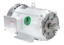
Leeson Washguard White Duck premium efficiency AC induction motor, washdown and inverter rated, 7-1/2hp, 3-phase, 230/460 VAC, 1800rpm, TEFC, NEMA 213TC frame, rolled steel, Cface/rigid base mount.
